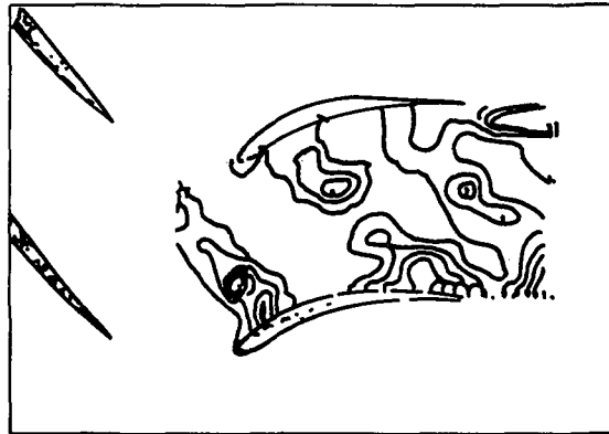
(a) Rotor trailing edge aligned circumferentially with stator leading edge.
