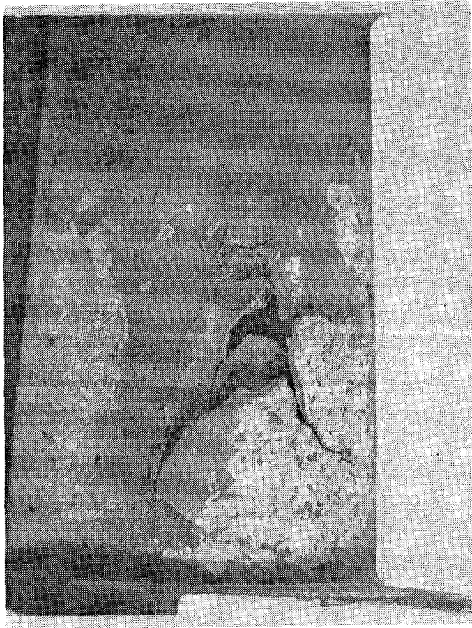
Figure 9. South American CF6-50 LPT Stage 1 Vanes After 15,155 Hours of Service.
