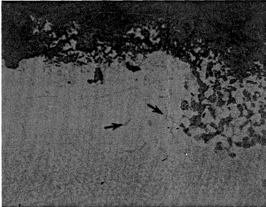
Figure 2. Southern Asia CF6-50 HPT Stage 1 Blade, Concave Side, 40%/80% Location, As Polished (1000×).
