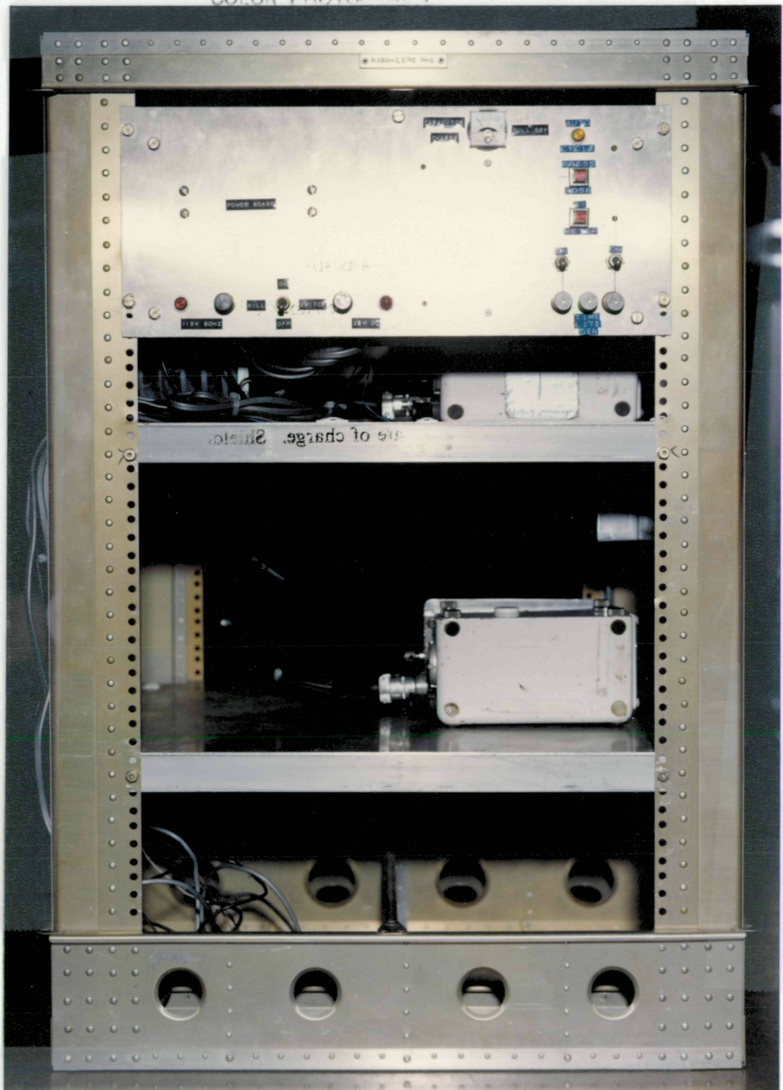
Figure 2-6. The automatic sequencing system. A photograph of the automatic sequencing system components installed in the NASA rack showing the control panel layout, and the two 16 mm movie cameras.
