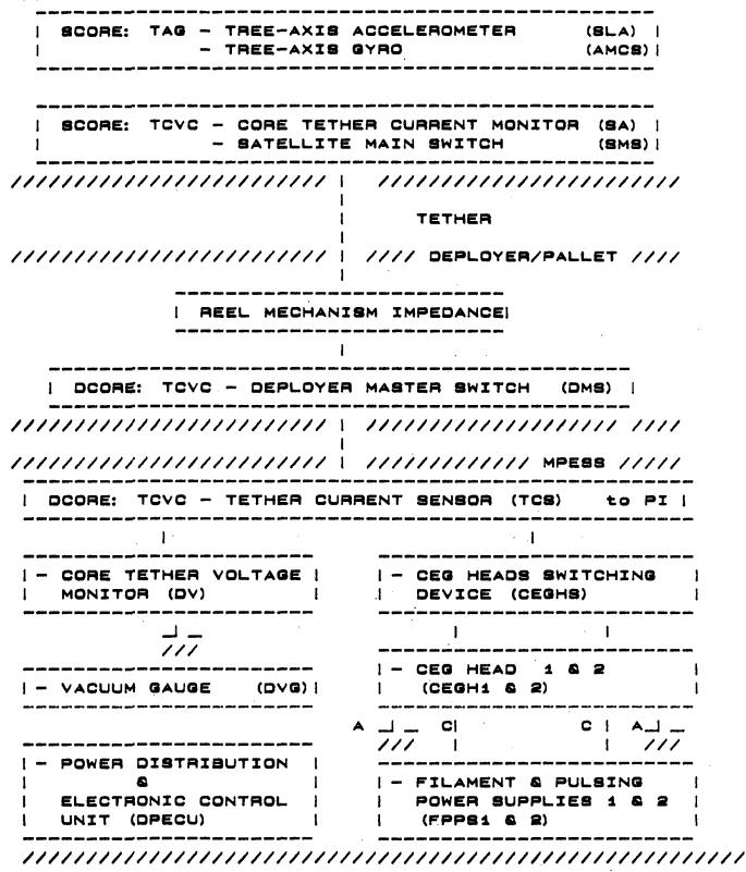
FIG.3.0-2 PSN/CNR PROVIDED CORE EQUIPMENT BLOCK DIAGRAM
