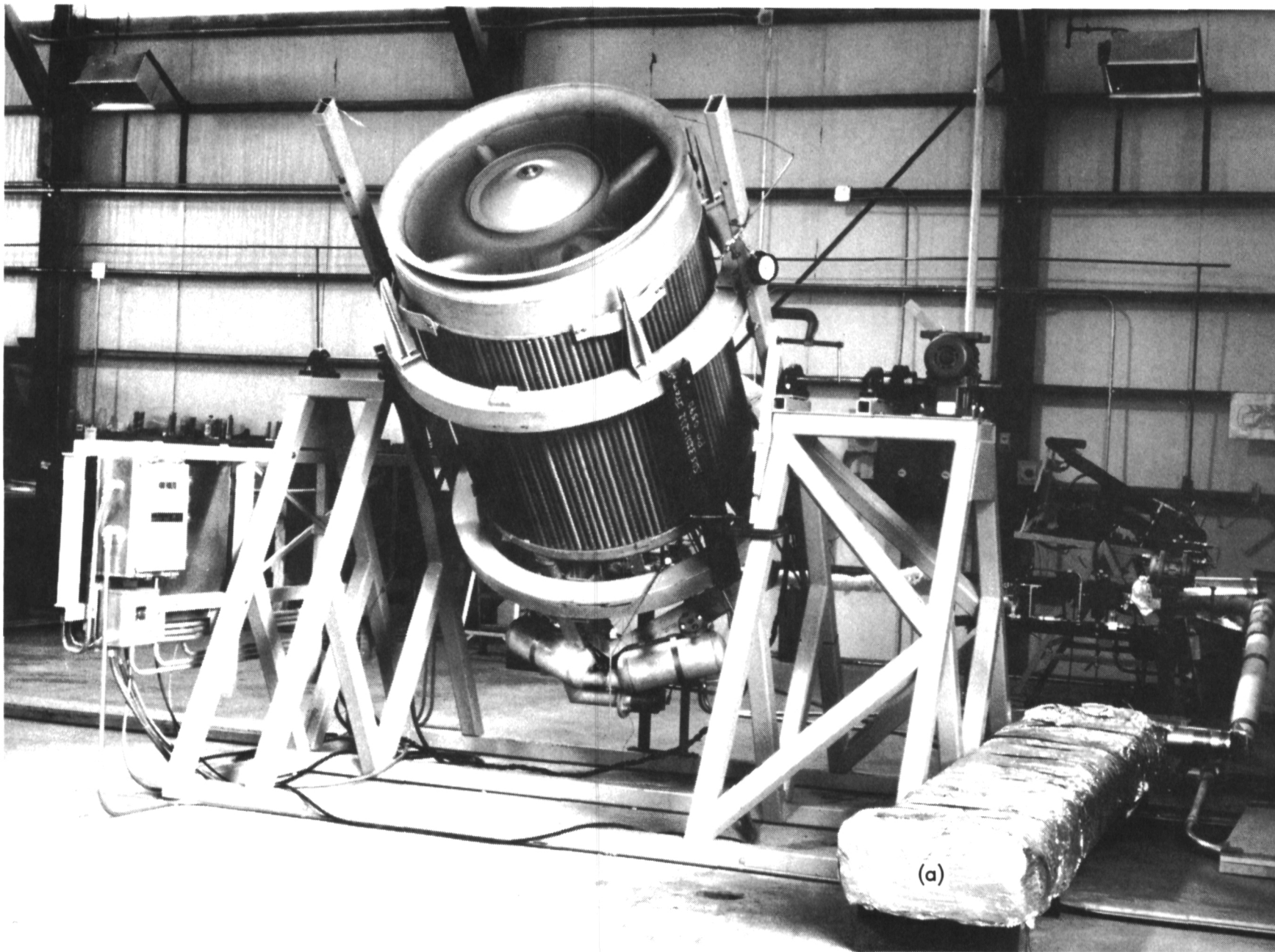
Figure 3-1. Power Conversion Subsystem Test at Barber-Nichols Using (a) an Electrical Resistance Toluene Vapor Generator
