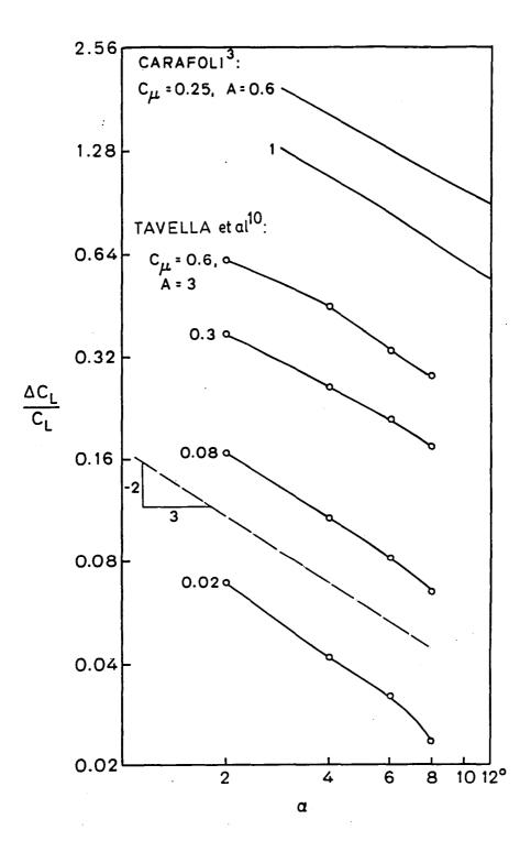
Fig. 7 Logarithmic plot of relative lift gain vs angle of attack.
