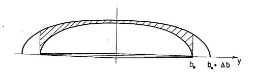
Fig. 2 The span perturbation concept: the shadowed region indicates lift gain.
