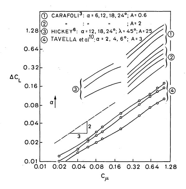
Fig. 6 Logarithmic plot of lift increment vs jet intensity
