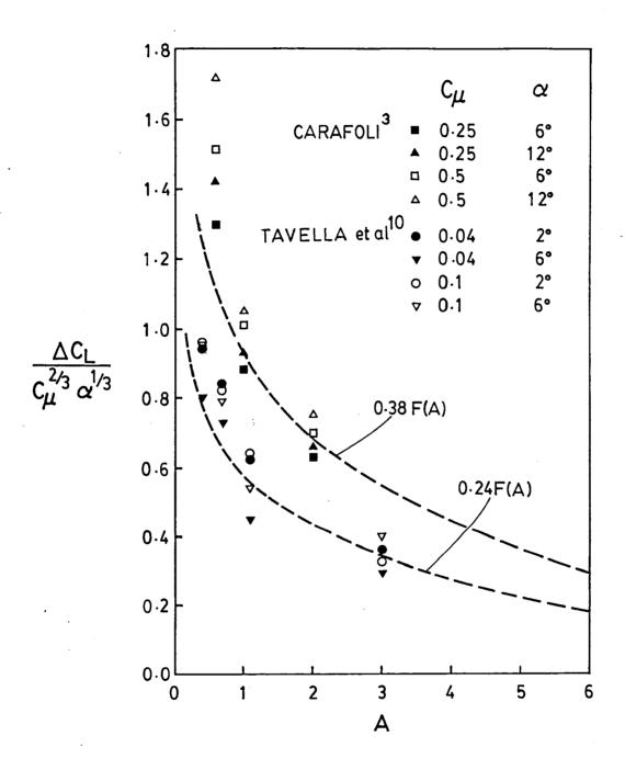
Fig. 9 Collapse of data for rectangular wings.
