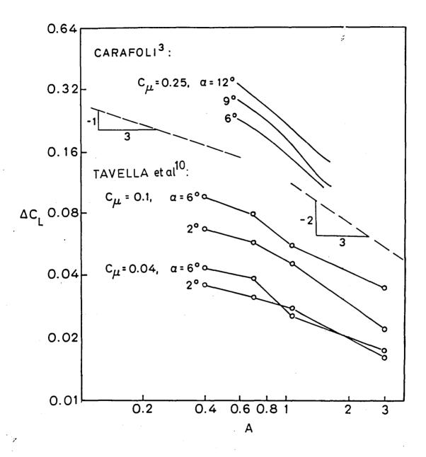
Fig. 8 Logarithmic plot of lift gain vs aspect ratio
