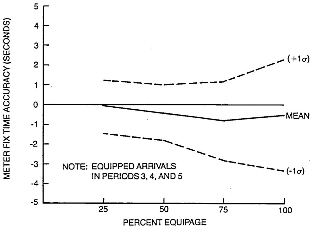
Figure 34 - Mean Meter Fix Arrival Time Accuracy vs Percent Equipage for Equipped Arrivals
