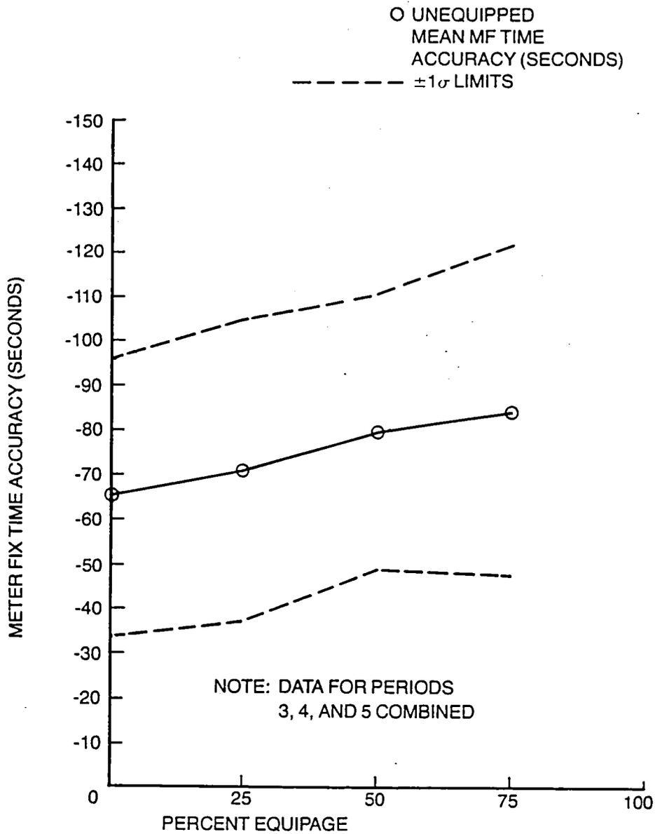
Figure 35 - Mean Meter Fix Arrival Time Accuracy vs Percent Equipage for Unequipped Arrivals
