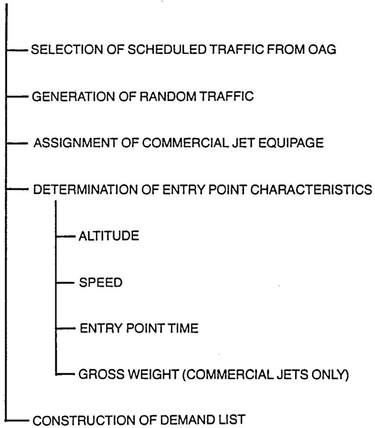
*Figure 18 - Traffic Model Functional Architecture*
