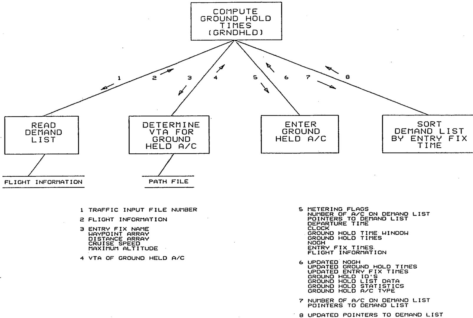
Figure 12 - Ground Hold Processing Module
