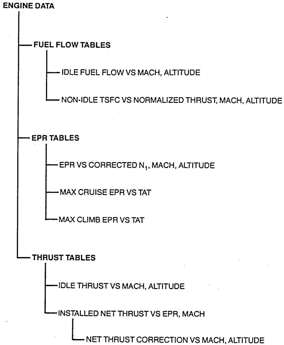
Figure 19 - Engine Data Base Architecture
