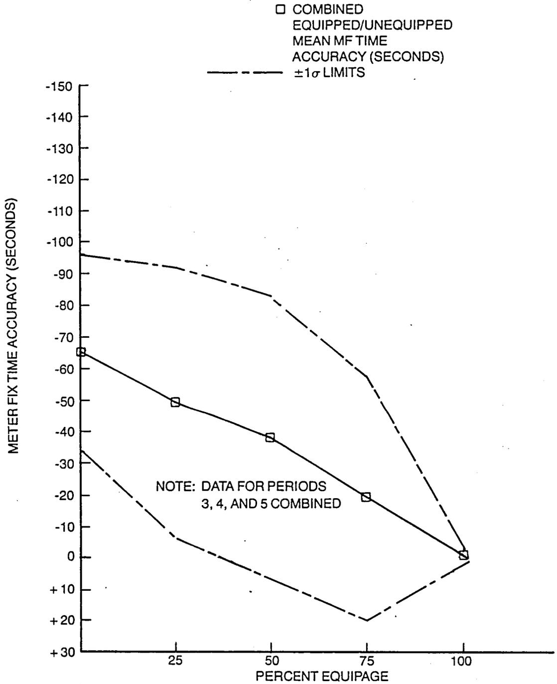
Figure 36 - Mean Meter Fix Arrival Time Accuracy vs Percent Equipage
