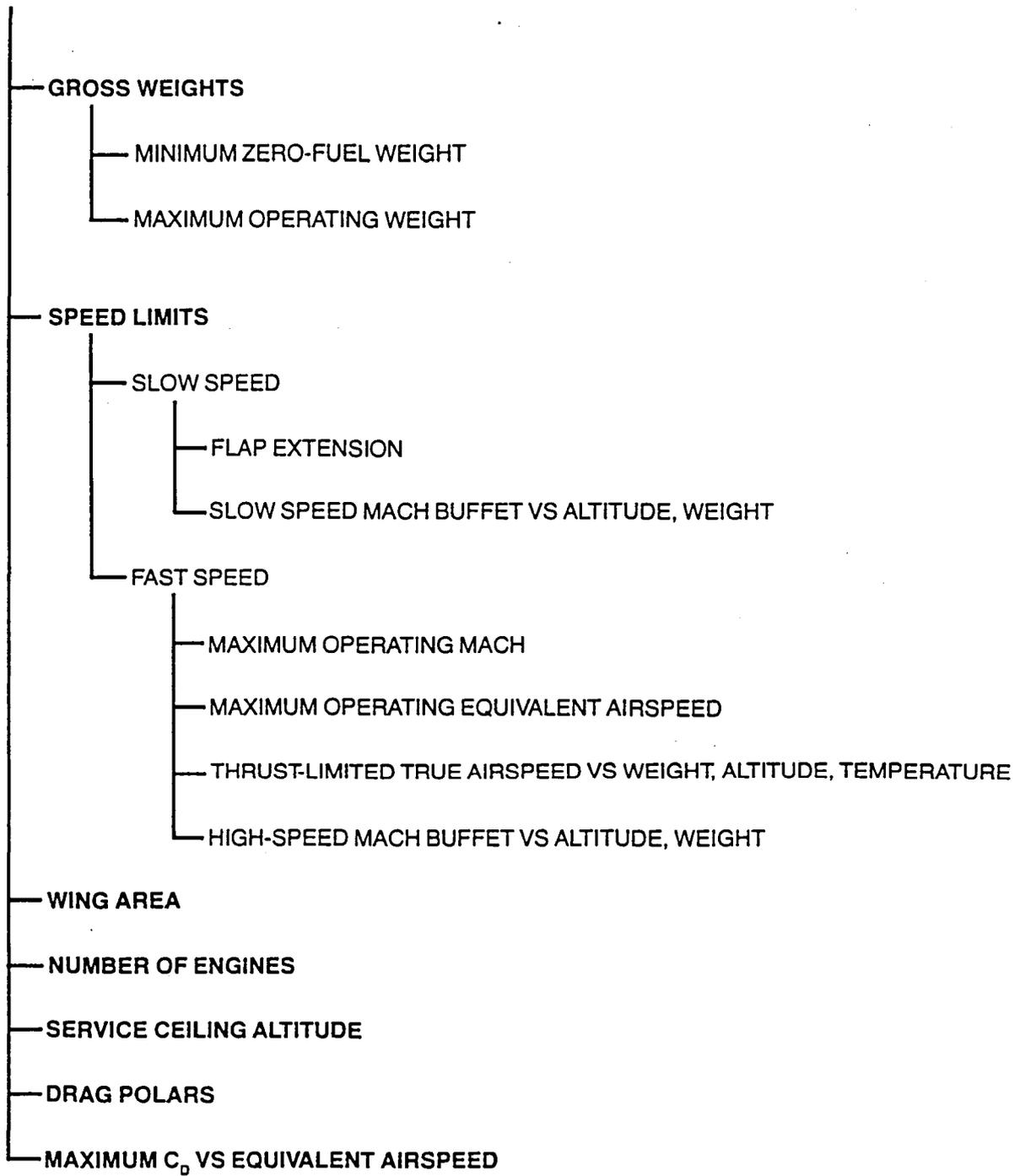
*Figure 20 - Airframe Data Base Architecture*
