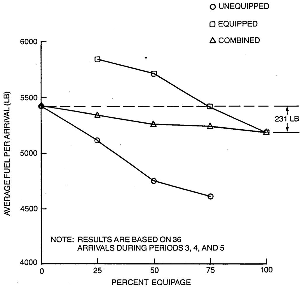
Figure 30 - Comparison of Equipped and Unequipped Average Fuel as a Function of Percent Equipage
