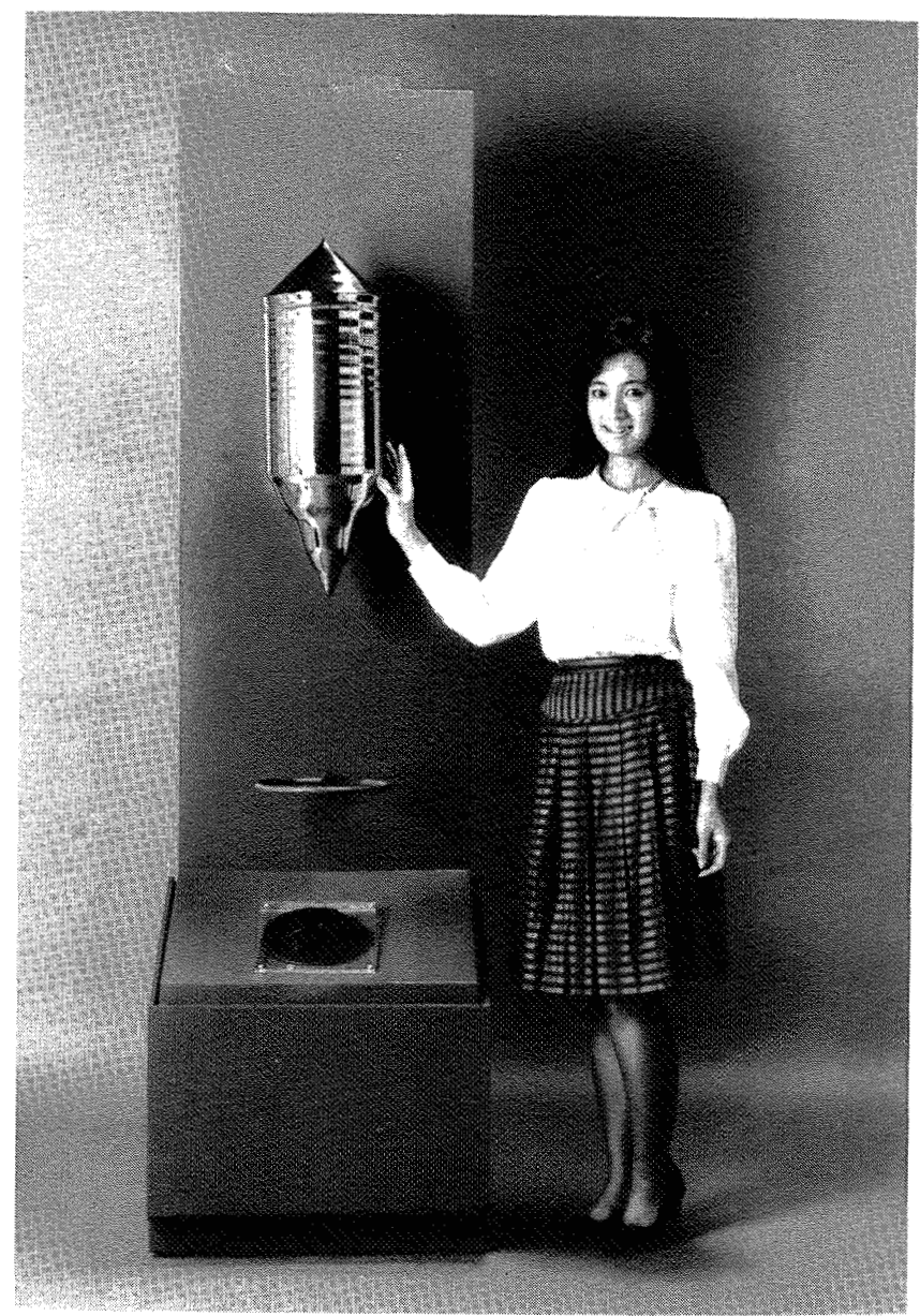
Cz Single Crystal, 250 mm in Diameter 45 kg in Weight
