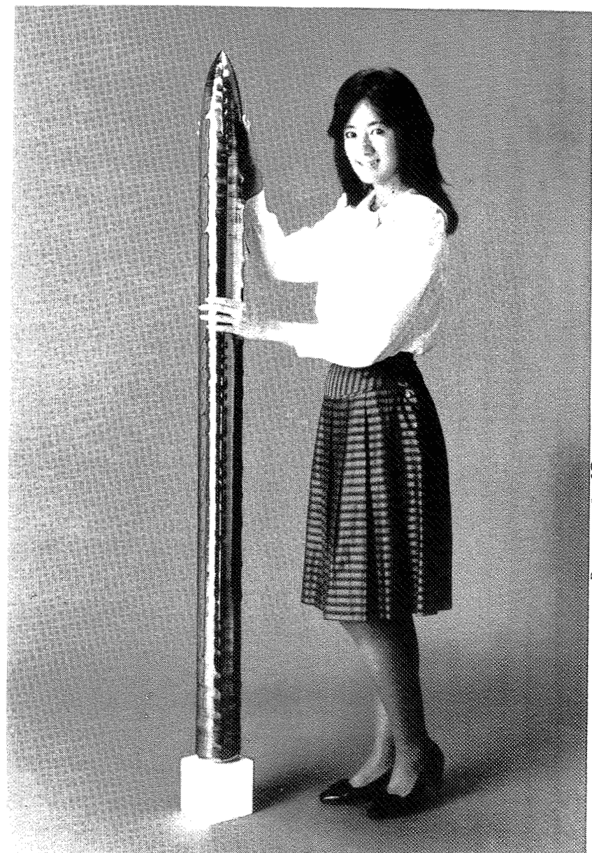
FZ Single Crystal, 100 mm in Diameter 1.6 m in Length
