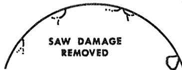
C. LAPPING, ETCHING AND POLISHING REMOVES SAW DAMAGE BUT NOT ALL OF THE GRINDING DAMAGE.
