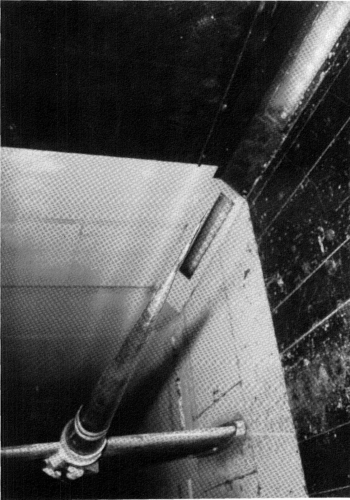
Figure 5. Single-probe configuration in 7 \times 10 HST.
