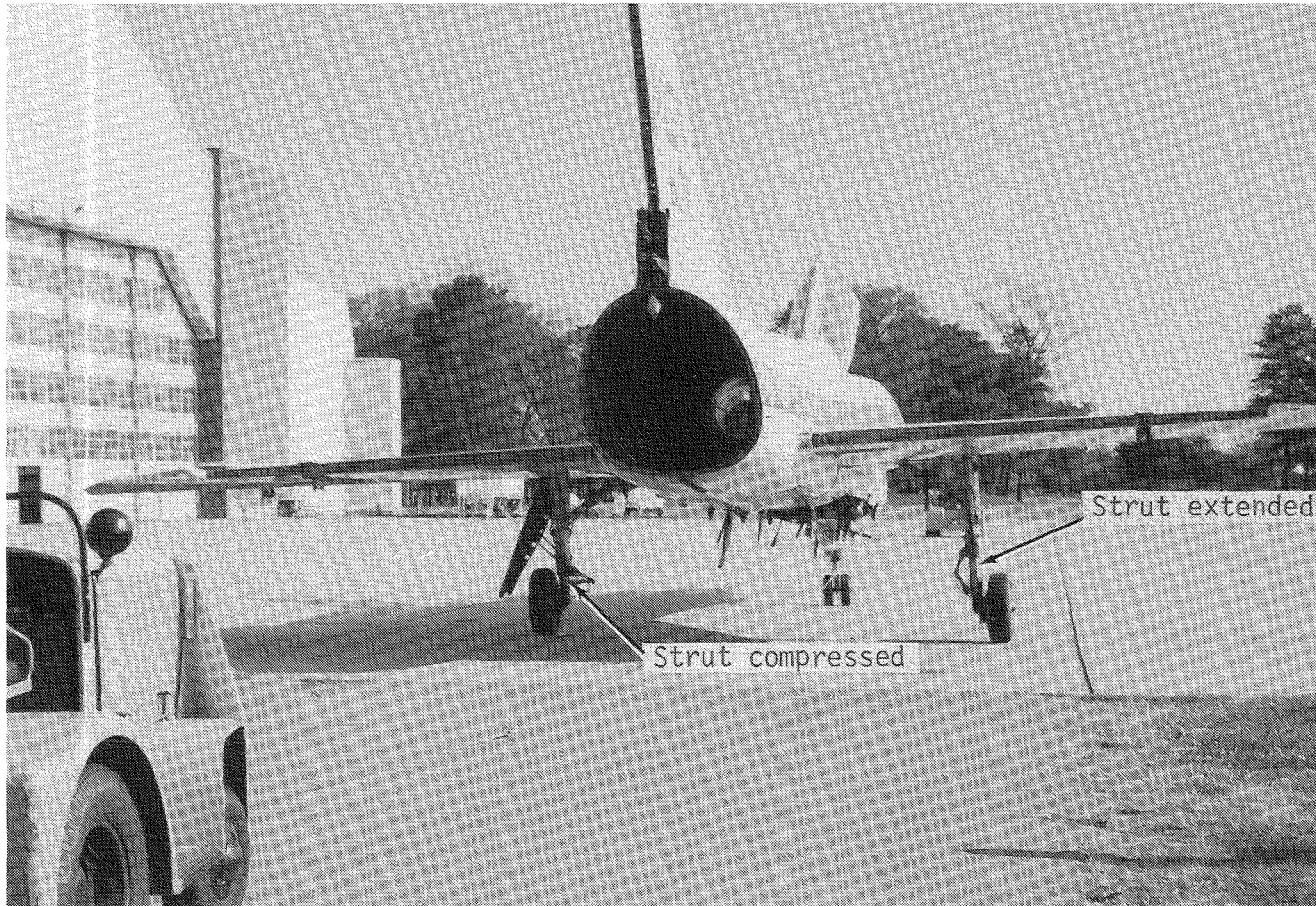
Figure 3. Differential strut strokes to produce bank angle of 3^\circ .
