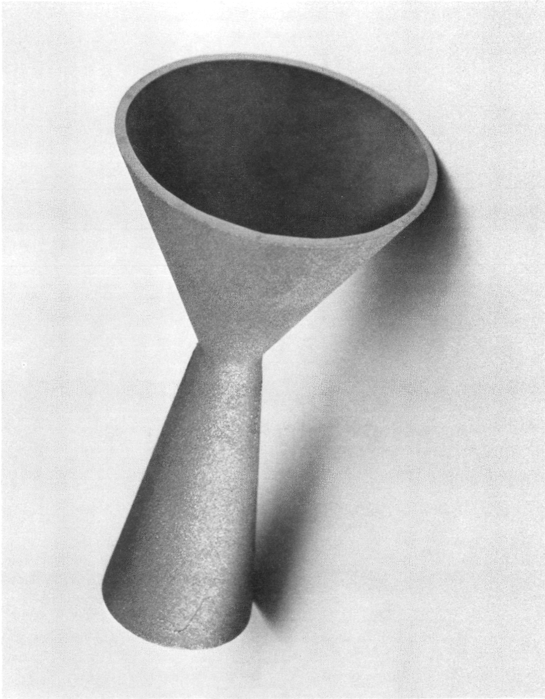
Figure 2.- Representative sample. Conical nozzle shapes of rhenium with metal oxide additives.
