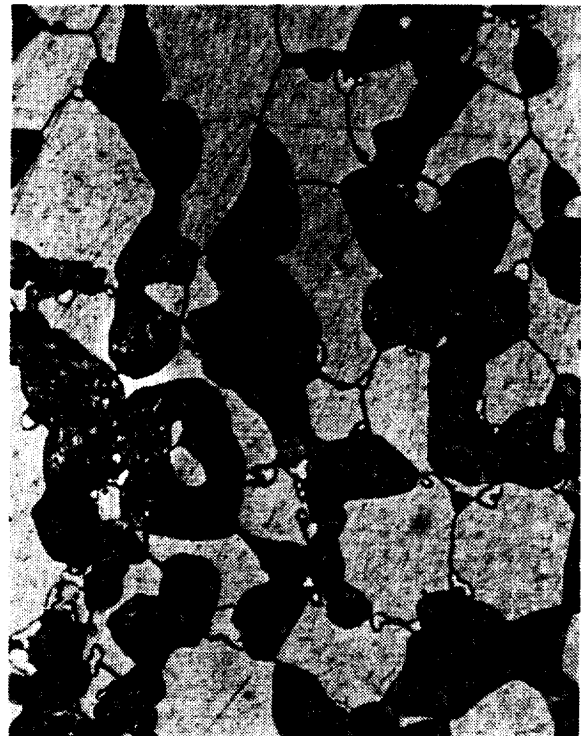
Etchant: Mod. Picral 500X Core (Hardness R_c 35)
