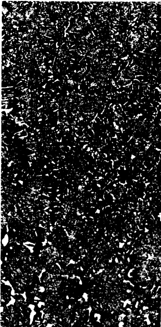
Etchant: Mod. Picral 500X Case (Hardness = R_c 63)
