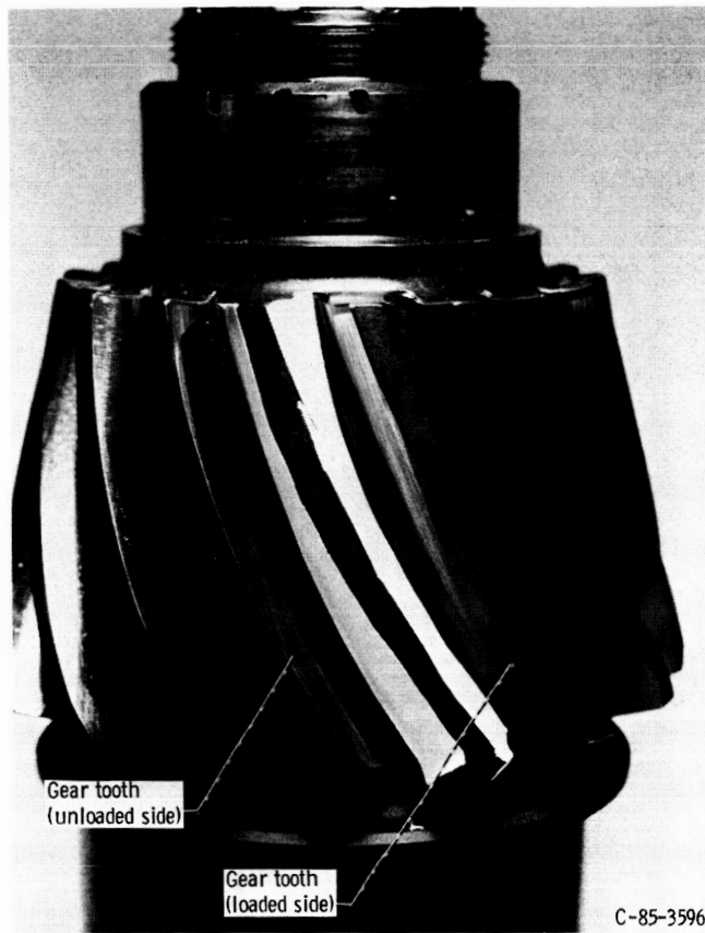
Figure 25.—Left spiral-bevel input pinion for UH-60A transmission.
