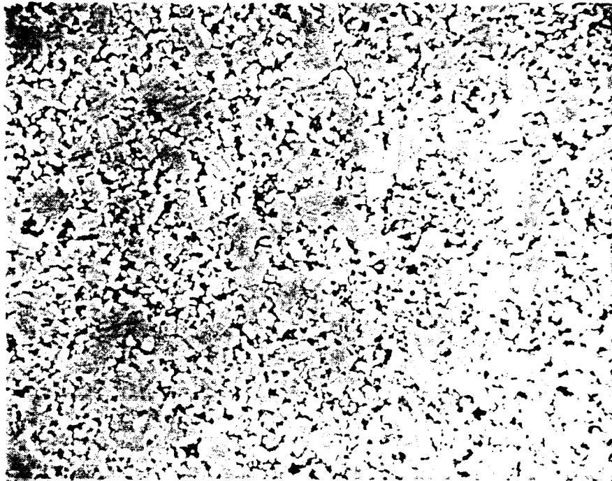
Figure 26. SEM of B doped SiC sample sintered at 1950°C for 1 hr in Ar. Magnification 9200X.
