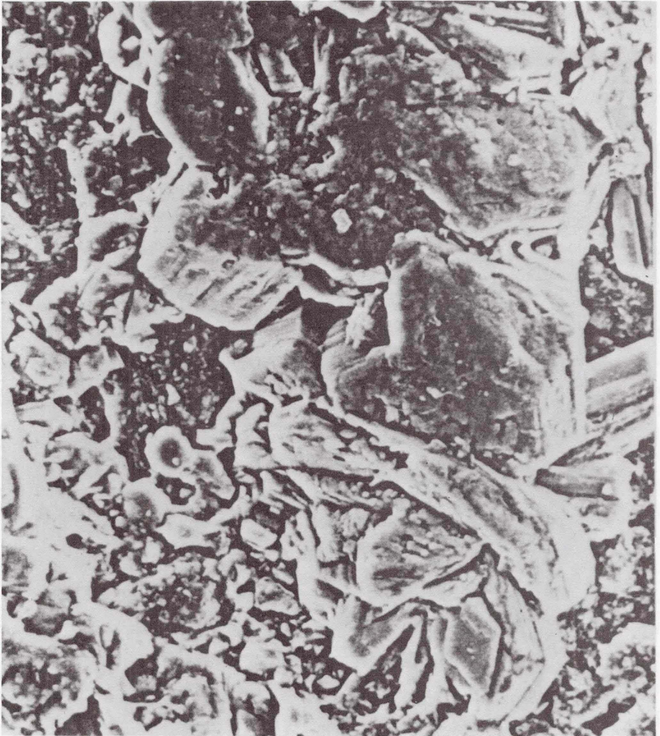
Figure 3. NaCr 2 O 7 CRYSTALS ATTACHED TO THE ELECTROLYTE SURFACE
