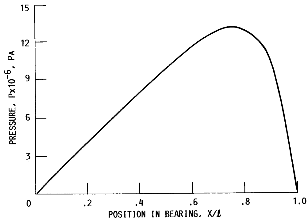
FIGURE 9.- PRESSURE VERSUS POSITION IN BEARING.
