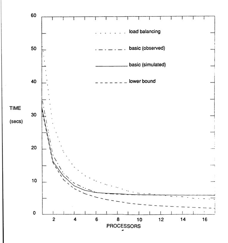
Fig. 11 Averages of observed timings of the two algorithms for N=1M compared with simulation and lower bound.
