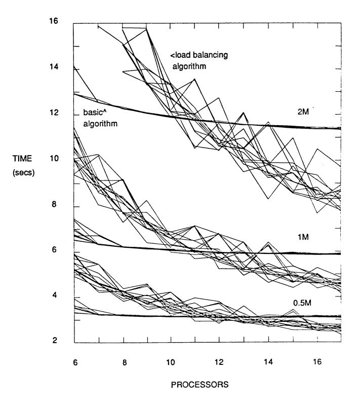
Fig. 10 Detail of plots of observed timings of Basic and Load Balancing algorithms for N=0.5M, 1M, 2M.
