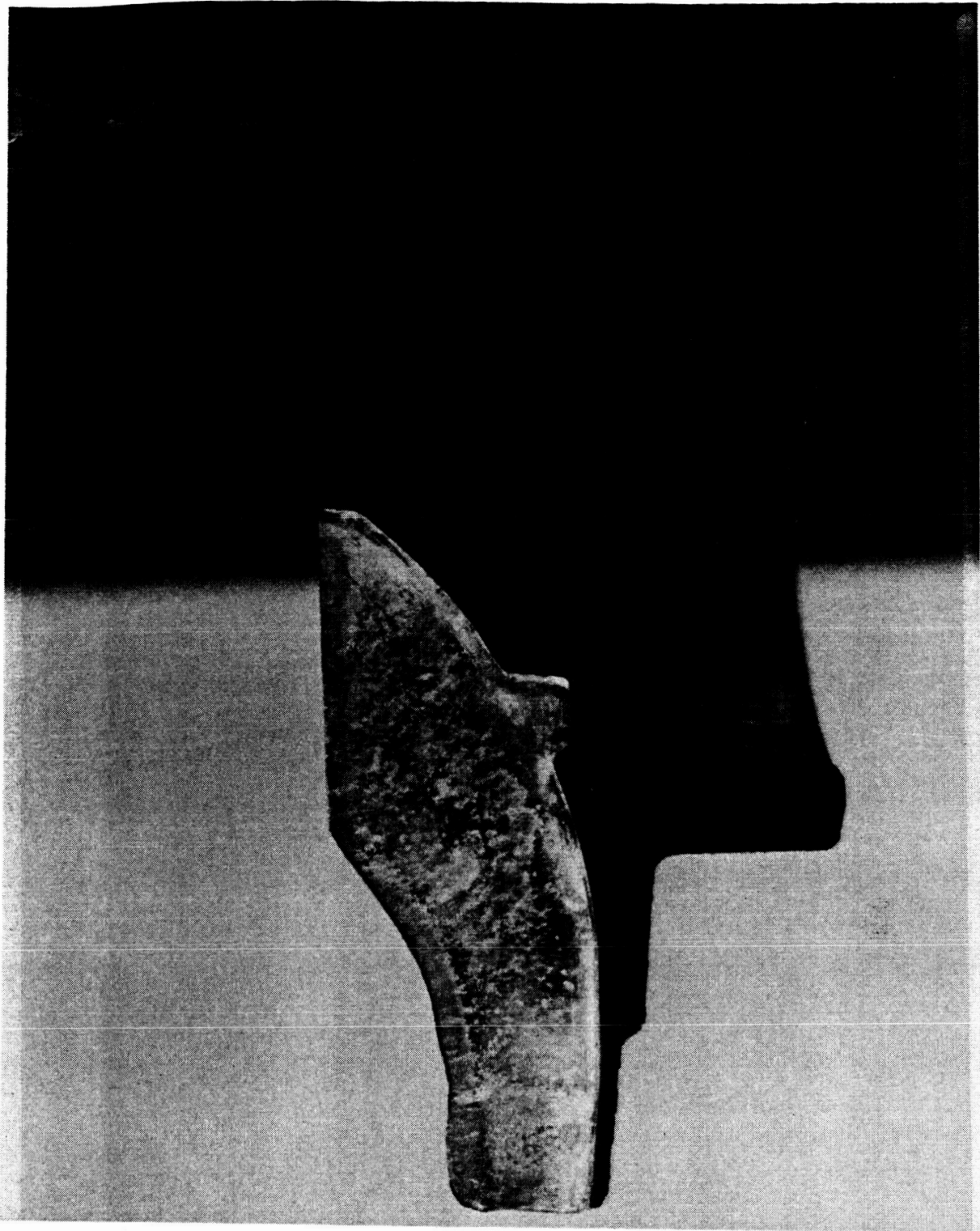
Figure 9B. Sectioned (Split) Blade Produced With Solid Core P/N 131103
