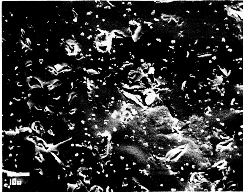
FIGURE 5. - MICROGRAPH TAKEN AT 1000X SHOWING A PARTICLE ERODED SURFACE AFTER 50 HOURS OF EXPOSURE TO THE OXYGEN PLASMA. THE APPEARANCE IS SIMILIAR TO THAT OF FIGURE 4. NO EVIDENCE OF UNDERCUTTING IS VISIBLE.
