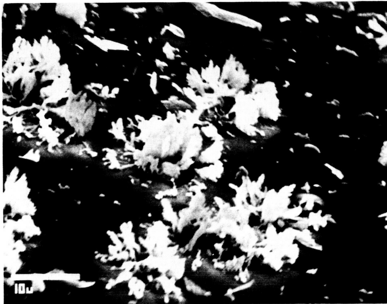
FIGURE 17. - MICROGRAPH OF THE SAME SAMPLE AS THAT OF FIGURE 16 AT THE SAME MAGNIFICATION AND A 60° TILT. OUTGROWTH OF OXIDIZED SILVER HAD BEEN CONTINUING AS OF 240 HOURS.
