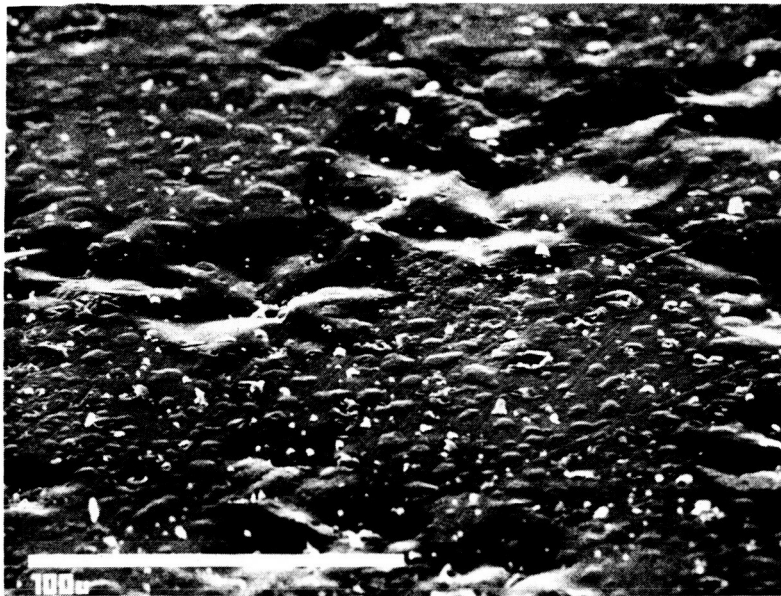
FIGURE 9. - MICROGRAPH TAKEN AT 500X OF THE LOWER RIGHT PORTION OF FIGURE 8 AT A SHARP ANGLE ( 60^{\circ} ) SHOWS THAT WHEREVER UNDERCUTTING HAD OCCURRED, THE SURFACE HAD COLLAPSED.
