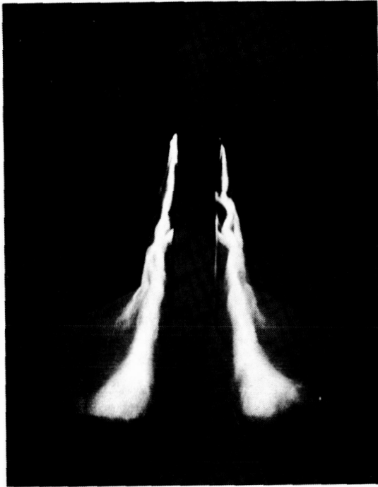
Figure 15. Vortex flows about YF-17 model at \alpha = 20^\circ (Northrop water tunnel).
