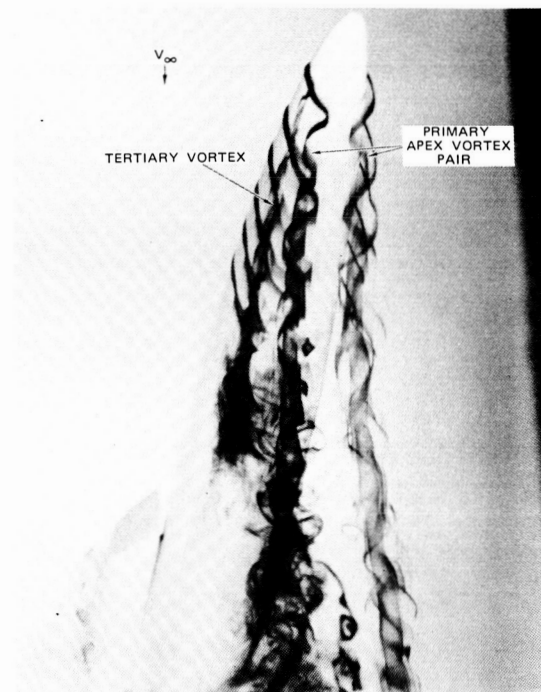
Figure 22. Close-up of vortex flows developed on forebody with shark nose (Northrop water tunnel).
