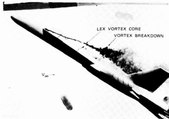
Figure 17. Vortex breakdown on a small-scale model of an advanced fighter configuration (Northrop water tunnel).
