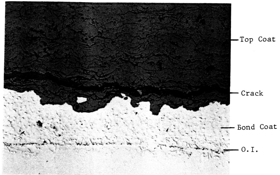
a) 100 hour argon pre-exposure ( 50 cycles )
