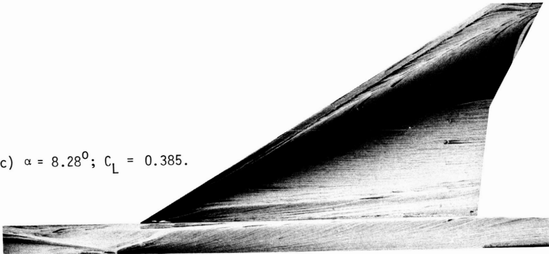
Figure B2.- Oil-flow photographs of 0/0/0/0 configuration. M = 0.5 .
