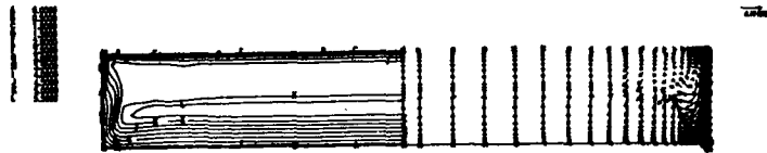
FIGURE 7.- MACH NUMBER CONTOURS AND SECONDARY VELOCITY VECTORS DOWNSTREAM OF COML LIP.
