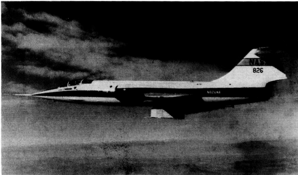
Figure 1. Flight test fixture installed on lower fuselage of F-104 carrier aircraft.
