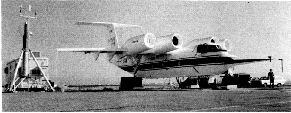
Figure 16.- Overall view of the QSRA installed on the load pads and the weather station.
