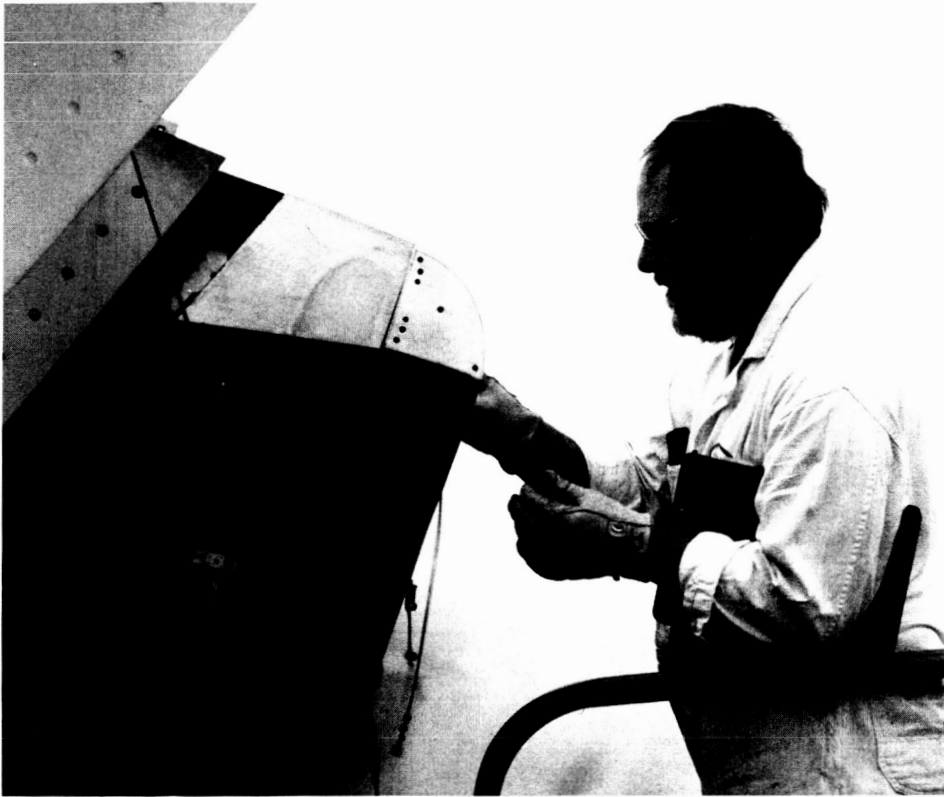
Figure 10.- End view of the 10-in.-diam, 90° arc CCW flap installed on the QSRA.
