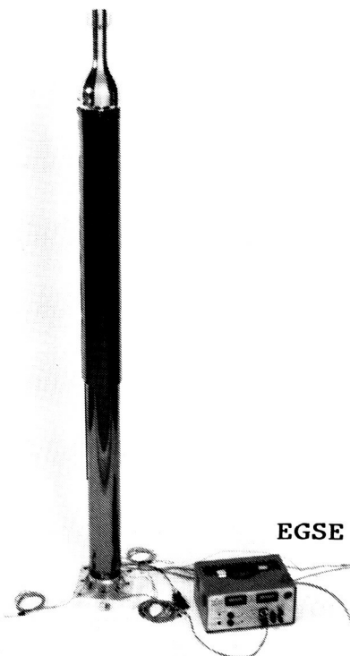
Figure 3. - S-Band antenna boom in deployed condition.
