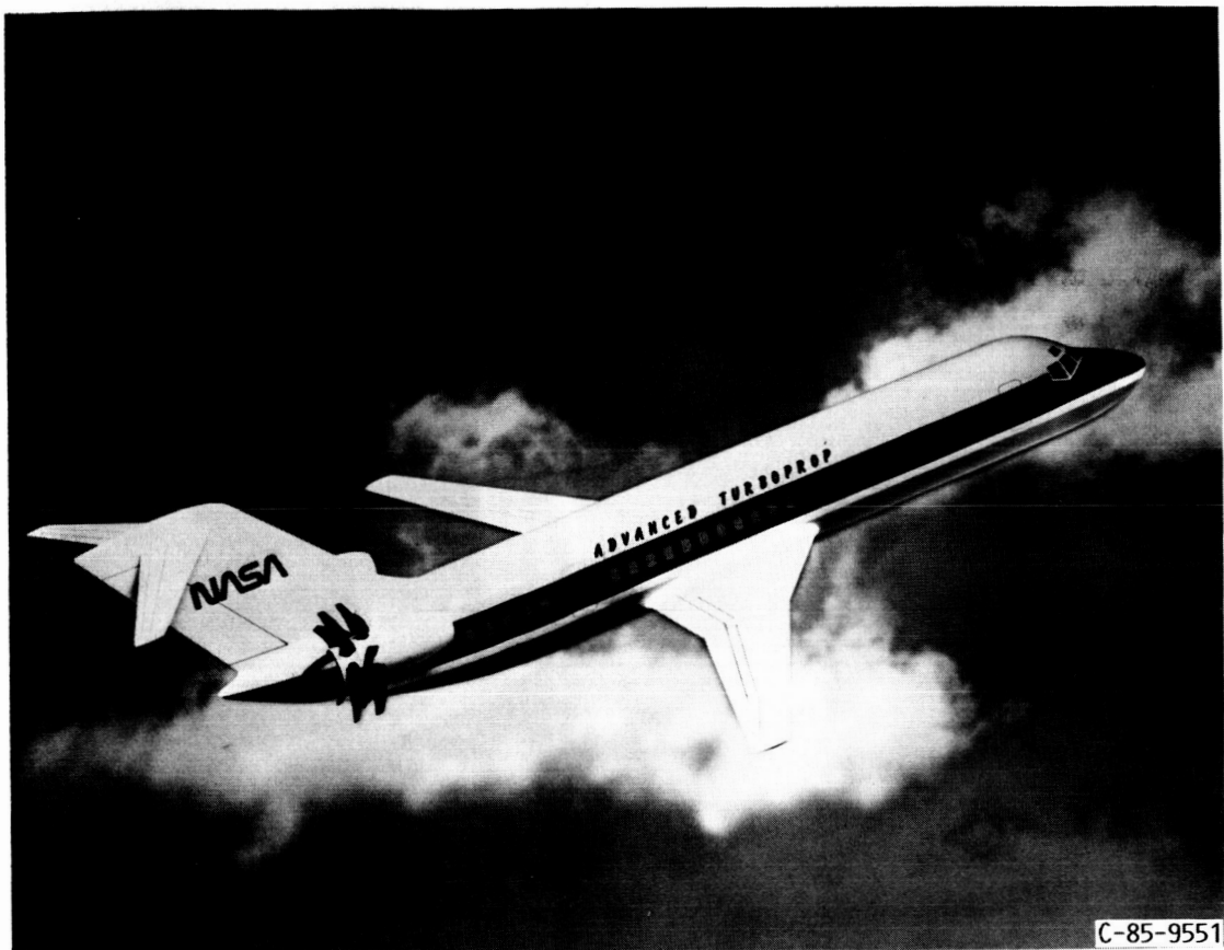
FIGURE 4. - G.E./NASA UDF AFT-MOUNTED PUSHER ENGINE INSTALLATION.
