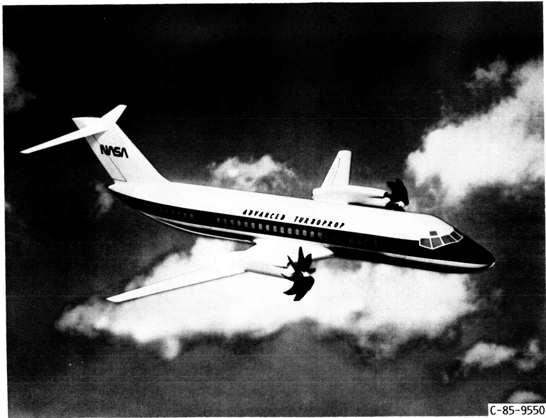
FIGURE 3. - WING-MOUNTED SINGLE ROTATION HIGH SPEED PROPELLER INSTALLATION.
