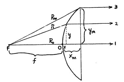
Figure 1. Illustration of a convex/plane convergent lens of focal length f and radius  $y_{m^*}$ . The thickness of the lens is  $x_{m^*}$ . An arbitrary ray follows a path in air of length R from the focal point F to a point on the front surface at coordinates (x,y) where it is refracted to follow a path parallel to the axis. The index of refraction of the lens material is n.
