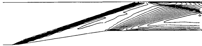
FIGURE 2. - MACH NUMBER CONTOURS FOR MACH 5 FLOW (ADAPTIVE DISSIPATION SCHEME).
