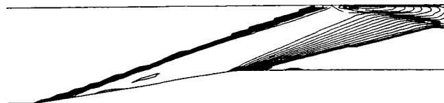
FIGURE 3. - MACH NUMBER CONTOURS FOR MACH 5 FLOW (PRESENT METHOD).
