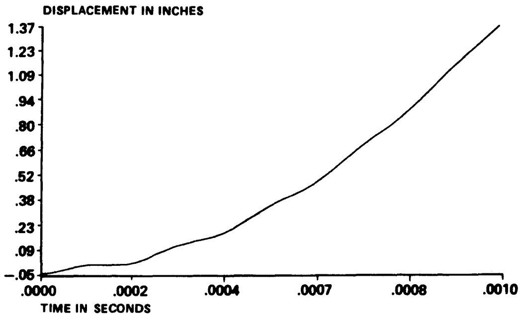
Figure 9. Response of free-floating O-ring compressed to 0.046 in. (linear elastic with pressure).
