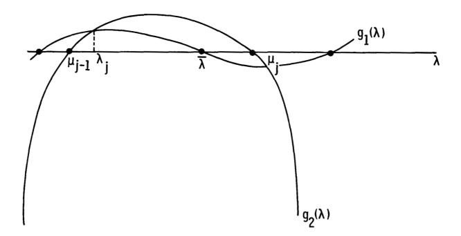
Figure 2. Schematic diagram showing roots of the cubic function of  $g_1(\lambda)$ , zeros of  $g_2(\lambda)$ , and  $\lambda_j$  where  $g_1(\lambda) = g_2(\lambda)$ .
