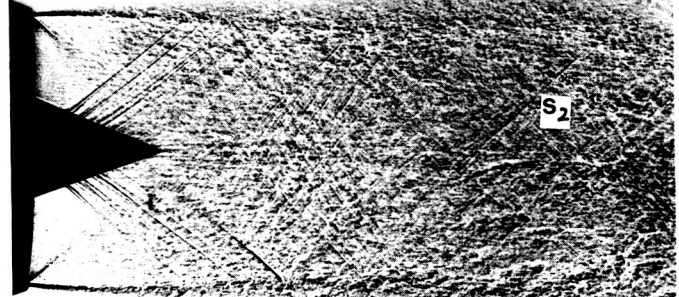
Porous Conical Plug-Nozzle ( \sigma = 4\% , holes locally distributed)
