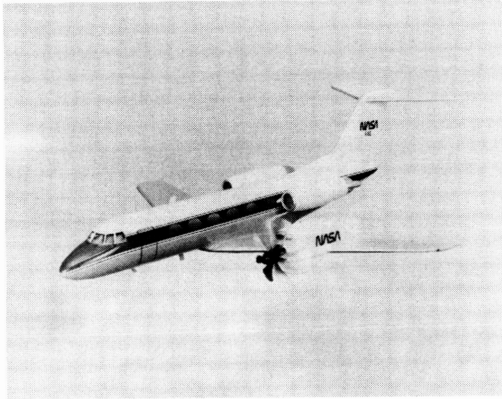
Figure 8 - Fuel-saving propfan mounted on the left wing of a Gulfstream II corporate jet (Lockheed-Georgia Company under contract to NASA Lewis Advanced Turboprop (ATP) Program).
