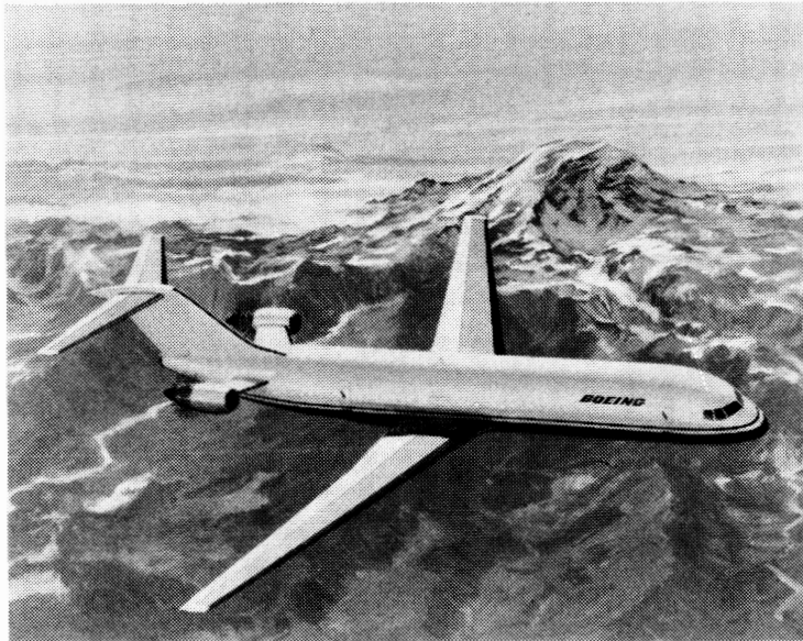
Figure 9 - 1990's advanced commercial airliner with advanced propfan, lightweight composite and lithium-aluminum alloys (Boeing).
