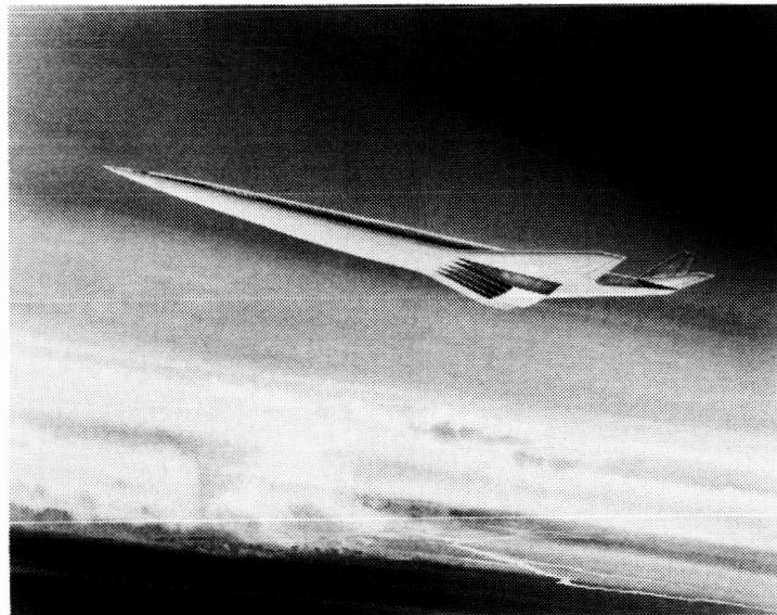
Figure 15 - Hypersonic passenger airliner (Lockheed/NASA) cruising speed 4000 mph, has propulsion system with both conventional turbojet engines and supersonic combustion ram (SCRAM) jet engines fueled by liquid hydrogen.
