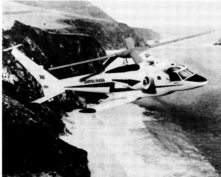
Figure 6 - DARPA/NASA/Sikorsky X-Wing concept has the vertical lift capability of helicopters while providing the range and speed abilities of fixed-wing aircraft. The X-Wing blades are made of graphite-epoxy composites and have a series of slots along their edges. Compressed air is blasted out of the slots to generate lift.
