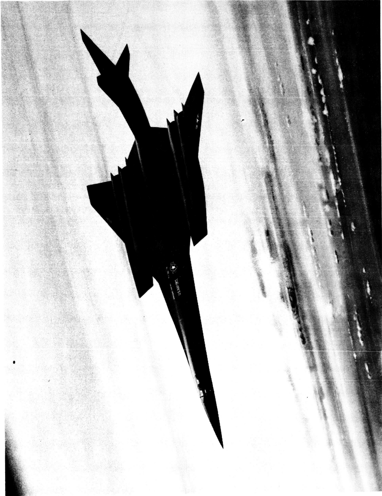
Figure 18.— Supersonic concept with thin, highly-swept surfaces.
