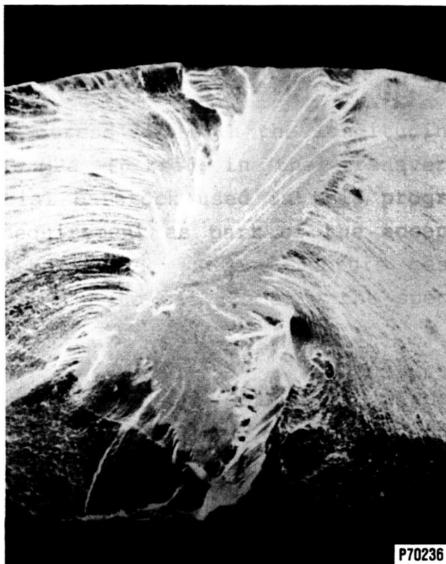
Figure 29. SEM Photos of HCF Specimen 604T-5 Fracture Surface, Showing Internal Initiation Site and Small Stage I Type Fatigue Associated with Origin Surrounded by Stage II Type Fatigue.
