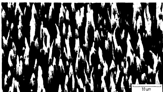
Figure 1.—Scanning electron microscope photomicrograph of fully developed textured carbon surface on copper substrate. Angle with surface, 30°.
