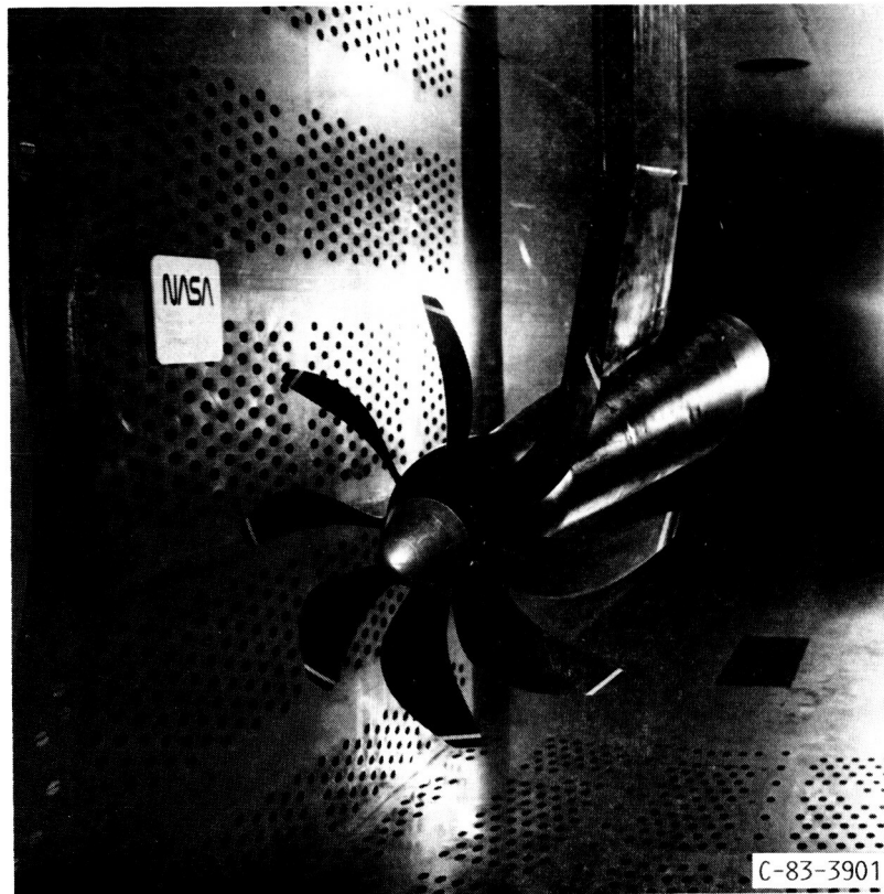
FIGURE 2.- SR3C-X2 PROPFAN MODEL WIND TUNNEL INSTALLATION.
