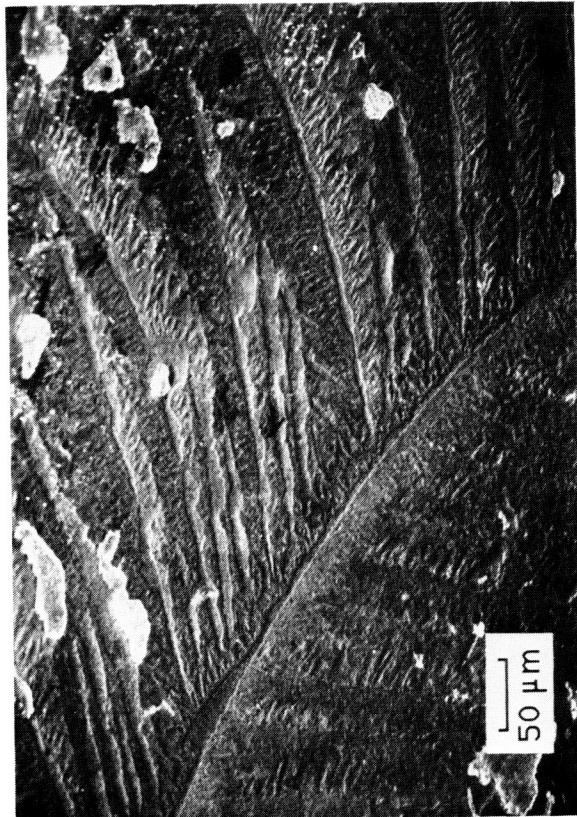
FIGURE 22. - TWO VIEWS OF DENDRITES ON SURFACE OF NICKEL-TIN EUTECTIC ALLOY FLIGHT SPECIMEN.
