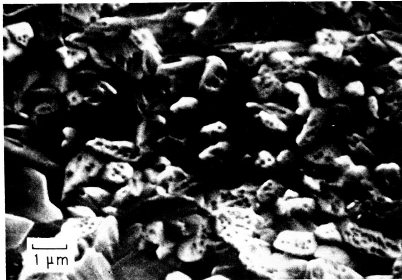
FIGURE 25. - FINE TWO-PHASE STRUCTURE ON THE FLIGHT SPECIMEN SURFACE.
