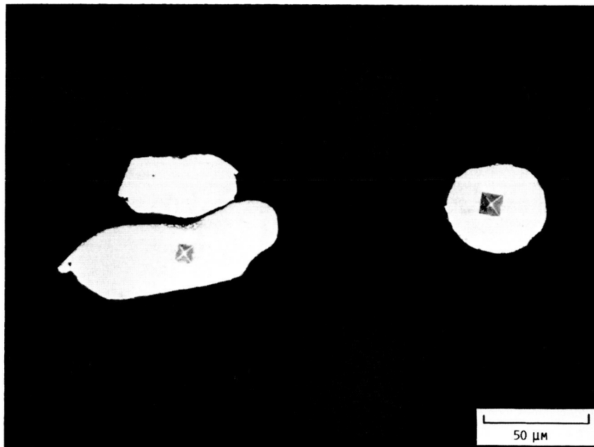
(B) MICROHARDNESS OF A DEFORMED WIRE (AT WIRE CROSSOVER) AND AN UNDEFORMED WIRE.
