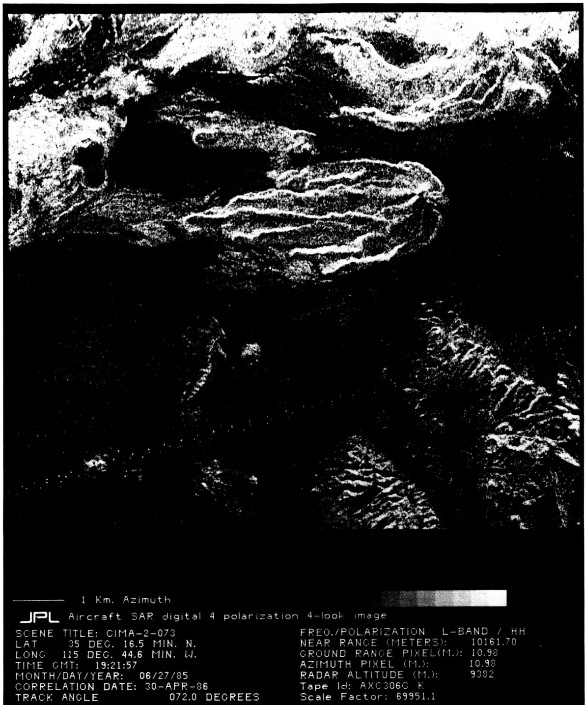
Figure 6-24. Digital HH Image of the Cima Volcanics Located in the Mojave Desert East of Los Angeles. There is little vegetation, so backscatter is controlled by slope and surface roughness. The bright area in the scene center is a young volcanic flow rougher than the adjacent sandy desert floor. Figure 6-20 shows the optical mosaic of this site. This scene is in the middle of the Figure 4-4 optical survey image.
