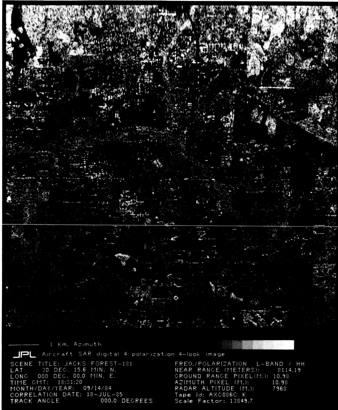
Figure 6-26. Digital HH Image of the Jacks Forest Site, Just West of Jacksonville, Florida. The bright areas are forested, and the dark stripe running top to bottom is an interstate highway where the pavement and shoulders reflect most radar energy away from the receivers on board the aircraft.
