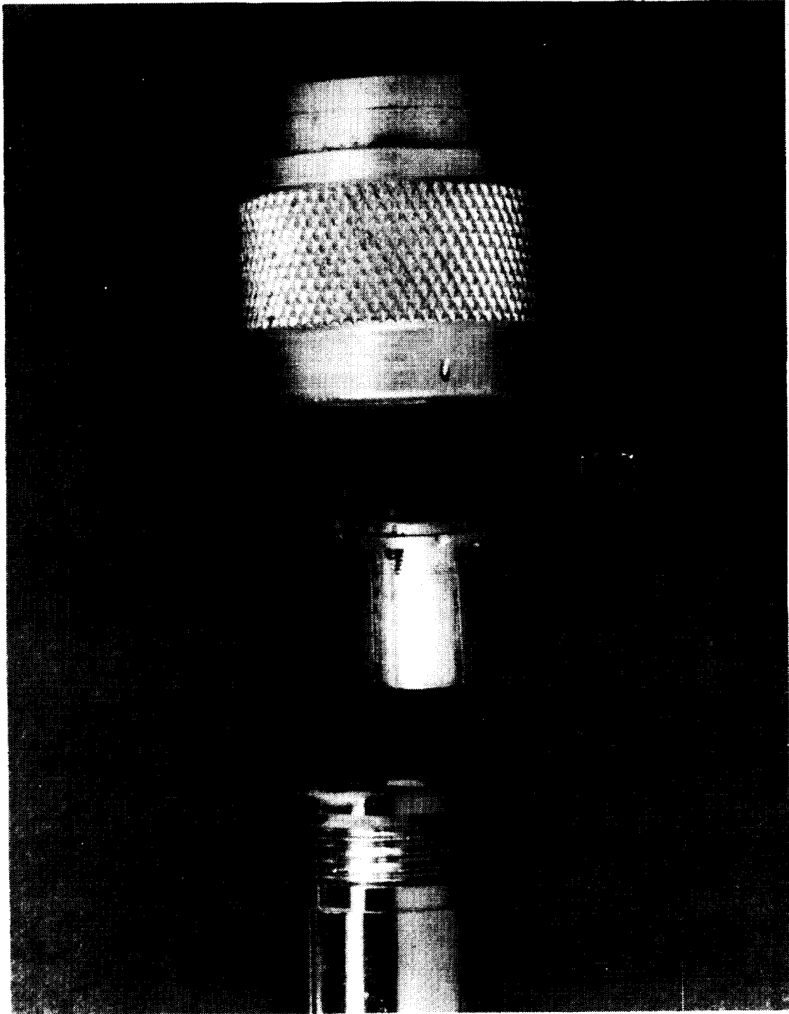
Figure 2-10. Special Capsule for Mounting Specimens of Capacitors Composed of Different Dielectric Materials. The Capsule Terminates a Sensitive Standing Wave Detector that could Resolve a Loss Tangent to Better than the Fourth Decimal Place, or the Difference Between 0.0026 and 0.0027, for Example.
