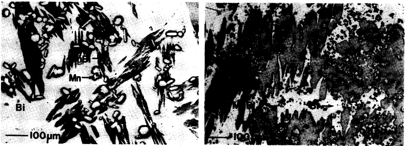
Fig. 3: Micrographs of Mn-Bi samples showing the distribution of Mn, Bi and the compound MnBi. Ground based sample left, flight sample right. MnBi compound is represented with grey color.
