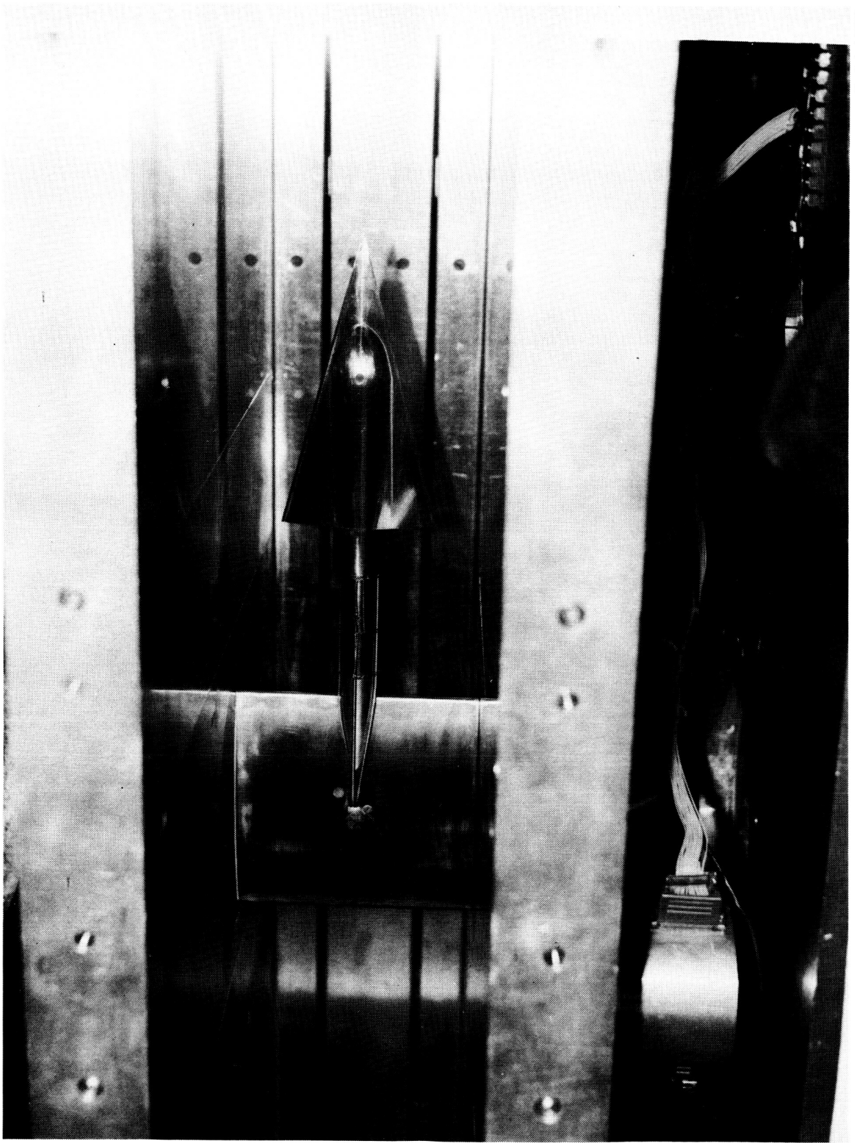
Figure 5. Top view of model, sting, and support strut in the Langley 0.3-m TCT.
