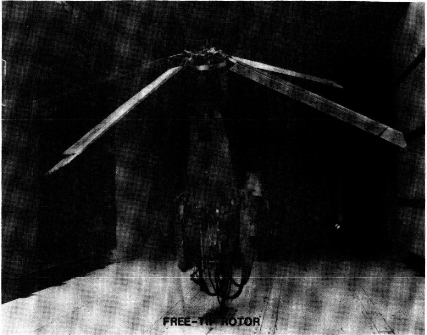
Figure 2.- Free-tip rotor in Boeing Vertol wind tunnel.
