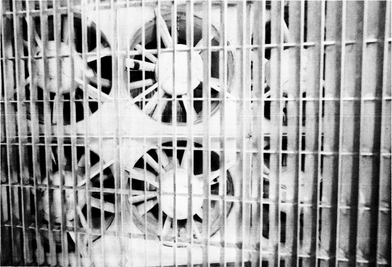
(a) One-fiftieth-scale model fan system as viewed through vane-set 5.
