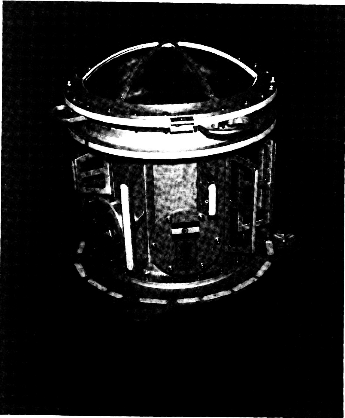
Figure 1. IONS payload flown in Space Shuttle Spacelab-3. In actual flight the payload was wrapped on its side by a thermal blanket for maintaining appropriate thermal environment and was placed on the open cargo bay on a specially mounted experiment support structure. The pressure inside the payload was maintained at 0.1 atm. during the flight with the help of pressure sensitive venting valves fixed on the wall of the payload.
