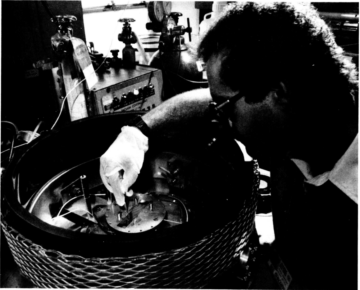
Figure 17. Photograph of a web cell being mounted for hydrogen ion implantation.
