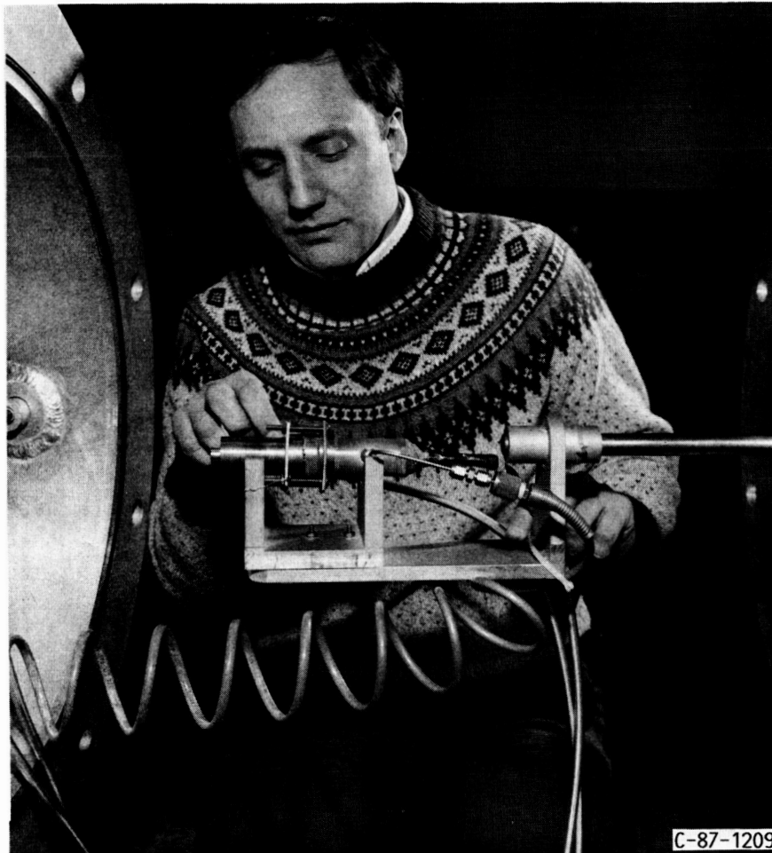
FIGURE 4. - PHOTOGRAPH OF ARCJET THRUSTER MOUNTED ON CRADLE ASSEMBLY.
