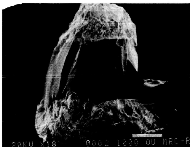
Figure 20. Pieces of flight sample 2 (35.7 CaO-39.3 Ga 2 O 3 -25 SiO 2 , mol%, hot pressed) showing the interior fracture surface examined by SEM. In A and C the crystalline region extended into the bulk ~1 mm from the imbedded platinum wire. The remaining portion of the bulk is glassy as shown in B and D. This sample is estimated to be 70 to 80% glass. A few small gas bubbles are visible in the center part of C and close to the bottom left side of the piece in D. Fracture surfaces were etched in 2% HNO 3 + HCl solution for 15 seconds at 25°C.
