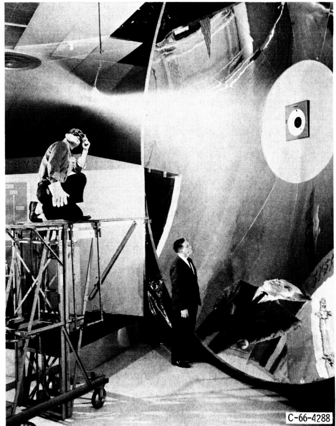
FIGURE 10. - AN EXPERIMENTAL PARABOLOIDAL SOLAR MIRROR 6 M IN DIAMETER.
